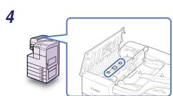
Clean the rollers (a total of three places) inside the inner cover with a water-moistened cloth. Then, wipe the area with a soft, dry cloth.
